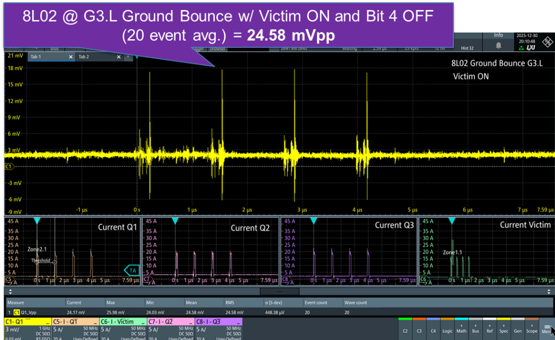
Figure 17 - Ground Bounce Measurement Result R3-8L-02 at G3.L with Victim Current ON and Q1 bit 4 OFF
