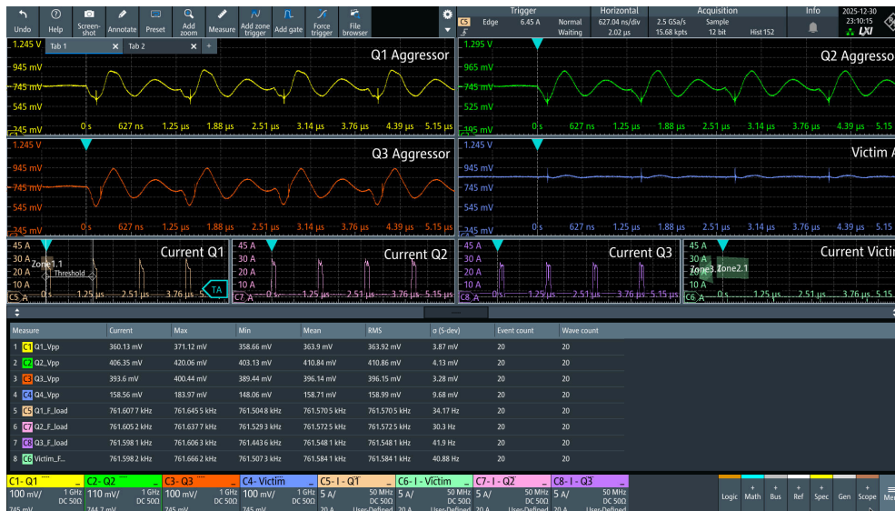
Appendix B - Worst-Case Crosstalk Amongst Test Cases With Victim Excitation Turned Off (R3-6L-01 with Victim Current OFF and Q1 bit 4 ON)
