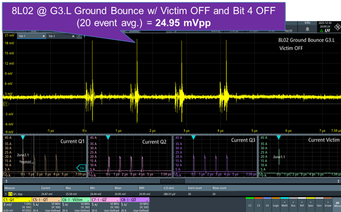
Figure 16 - Ground Bounce Measurement Result R3-8L-02 at G3.L with Victim Current OFF and Q1 bit 4 OFF
