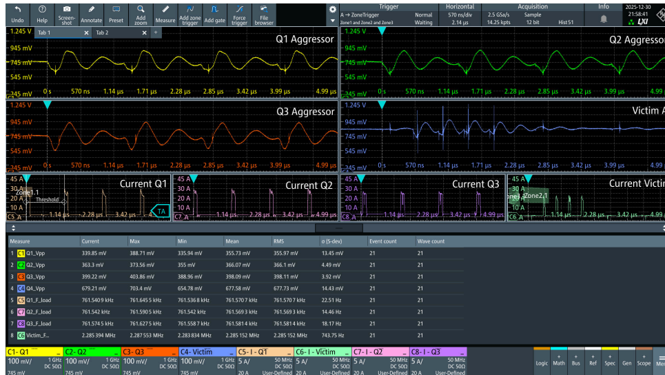
Appendix A - Worst-Case Crosstalk Amongst All Test Cases (R3-6L-01 with Victim Current ON and Q1 bit 4 ON)
