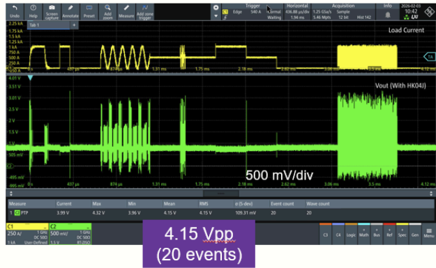
Figure 20 - Measured Voltage Responses to 1000 A Dynamic Loads (Yellow/top: Current, Green/bottom: Voltage)
