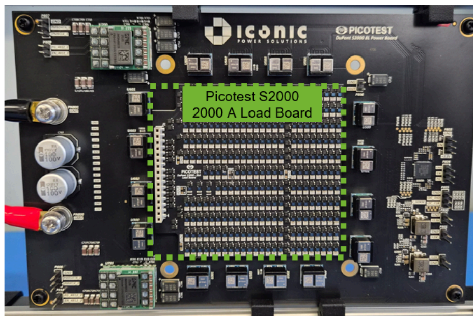
Figure 4 - Test Fixture with Load Board Mounted on Power Board
