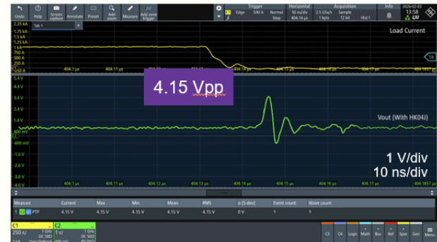
Figure 21 - Measured 1000 A to 0 A Step Response (Yellow/top: Current, Green/bottom: Voltage)
