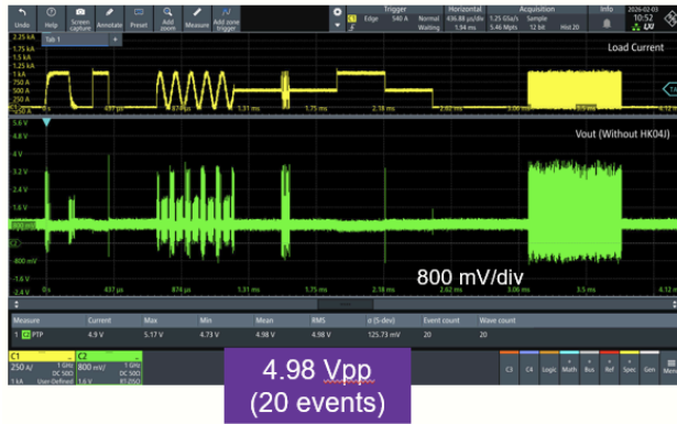
Figure 20 - Measured Voltage Responses to 1000 A Dynamic Loads (Yellow/top: Current, Green/bottom: Voltage)
