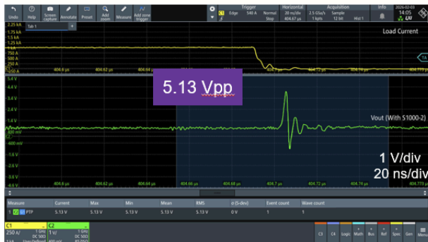
Figure 21 - Measured 1000 A to 0 A Step Response (Yellow/top: Current, Green/bottom: Voltage)
